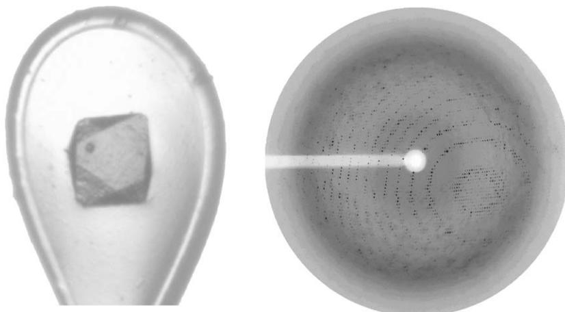
Fig. 1. A protein crystal mounted and frozen within a cryo-loop and the resulting X-ray diffraction pattern recorded at a synchrotron source. Images courtesy S. Törnroth.
